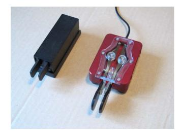
Unlike the Palm Mini there are no magnets in the bottom of the lightweight mechanism.
