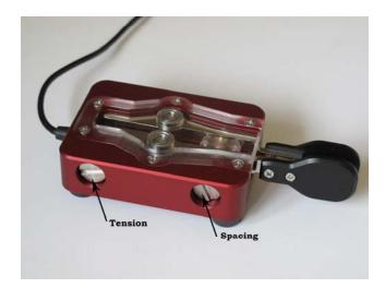
Adjustment of spacing and tension is done via two large bolt heads on each side of the paddle mechanism, which are locked in position by small grub screws on the underside.
